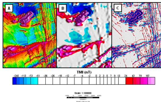
Figure 4: Plots of total magnetic field from Iroquois Falls region. A) Original TMI dataset gridded at 20m. B) Regional TMI dataset gridded at 640m. C) Residual TMI dataset produced by the subtraction of B) from A).
