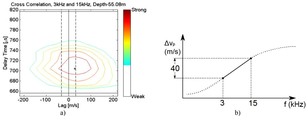
Figure 3: a) Cross correlation of semblance plots in Figure 2a and 2b. Velocity lag of about 40 m/s is observed. Weak correlations are shown in white. The asterisk “\*” indicates correlation value computed from the maximum correlation method. b) P-wave velocity dispersion graph obtained from a). Dotted line shows predicted trend by Pride (2005).
